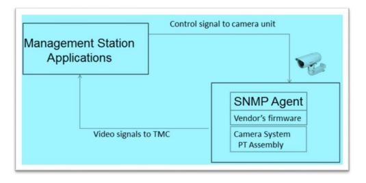
Figure 1: CCTV System Communications Interface
