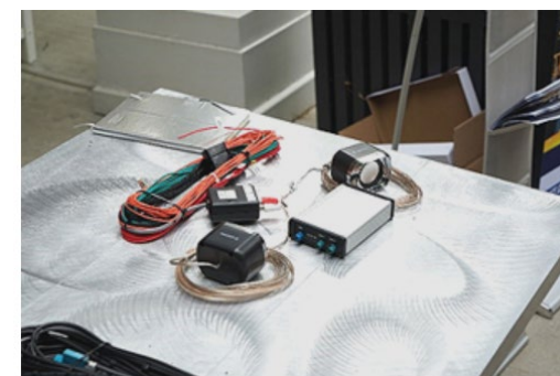
CV equipment, including the ASD and pair of speakers, prior to installation in the NYCDOT vehicle. Source: NYCDOT
