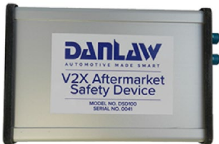
Danlaw V2X ASD being installed in the participant vehicles of the NYCDOT CV Pilot
