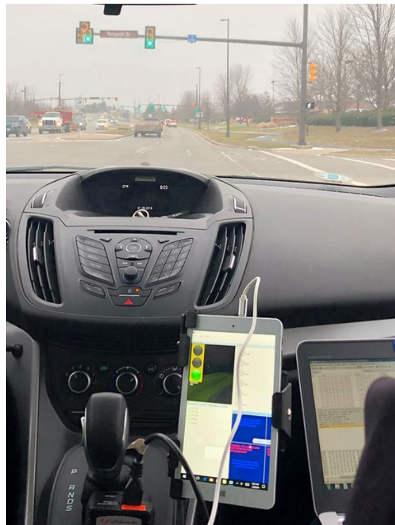
On-board unit installed in City of Dublin vehicle
