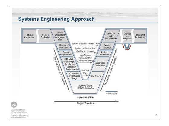
This figure represents the systems engineering process in the shape of the letter "V." The project timeline and process flow run from the upper left, down to the point of the V, and up to the right.
